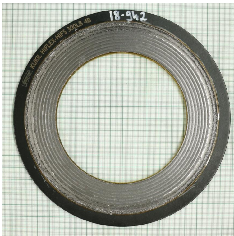
Shell leakage test (RT) according MESC SPE 85/300 - 3.3.2
