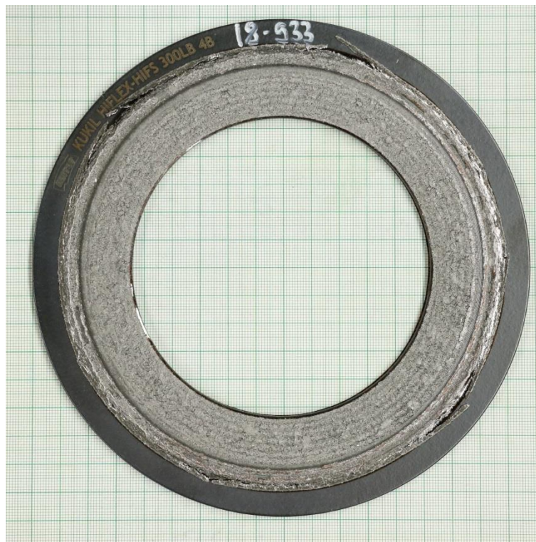
Shell cycle test (T) according MESC SPE 85/300 - 3.3.5
